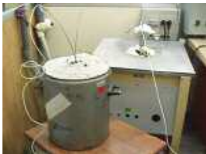
Calibration by comparison: salted bath
